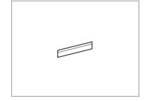
Rectified edges. Recommended joint 1 mm
